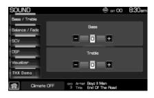
**Balance/Fade:** Press to adjust the sound between the left and right speakers (Balance) and to adjust the sound to the front and rear speakers (Fade).
